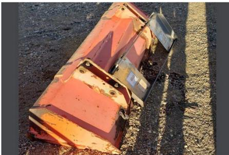
This is a photo of the bucket with the weld-on plate lying next to it. Some buckets (like this one) have a brace across the back. You may need to remove some of the brace to accommodate the length of the weld-on plate, but leave as much as you can to maintain the structural rigidity of the bucket.
