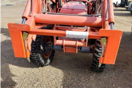
When you're changing from a pin-on bucket to quick attach, the first step is easy if the bucket pins have been greased on a regular basis. Put the tractor on a level surface and remove the pins that hold the bucket on. Back the tractor up while not changing the height or angle of the loader arms. Position the quick attach faceplate where the bucket was and reinstall the pins. It helps to have two people working on this project.
