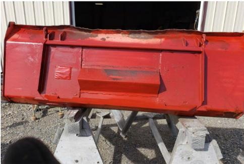
With the welding done, it's time to shoot some paint on the new bracket and the back of the bucket to prevent rust and oxidation.
